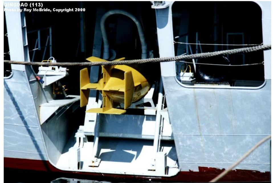
Both Type 052 Luhu class destroyers, *Harbin* (112) and *Qingdao* (113), were fitted with the U.S. designed DE-1164 integrated hull sonar and variable depth sonar (VDS), not the French DUBV-23/43 as reported in Jane's publications.
