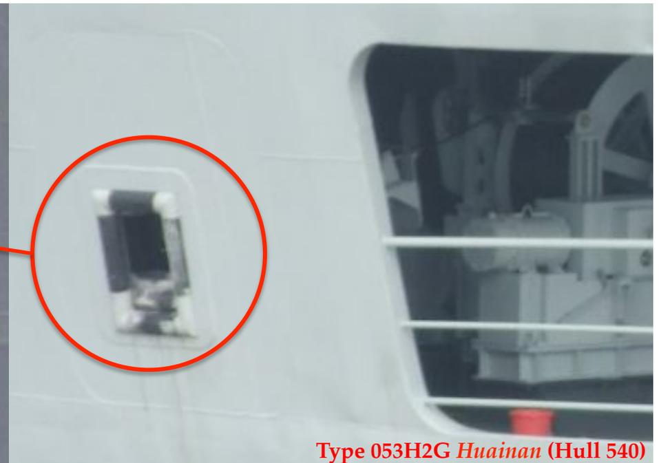
The towed array deployment port on Type 054A Flight II ships is virtually identical with the one found on the Type 053H2G JIANGWEI I frigates *Huainan* (Hull 540) and *Tongling* (Hull 542). This strengthens the argument that the ports share the same function.
