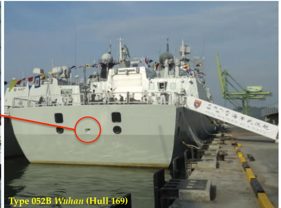
The configuration of the Type 054A Flight II frigates can also serve as an indicator for other PLAN ships. Case in point, all Type 052C destroyers have a very similar stern arrangement with a towed decoy opening to port and a towed array opening to starboard. The Type 052B destroyers only have a towed decoy opening at the center of the transom. From this it can be concluded that the Type 052B DDGs *will not* be fitted with a towed array, while the Type 052C will have one.
