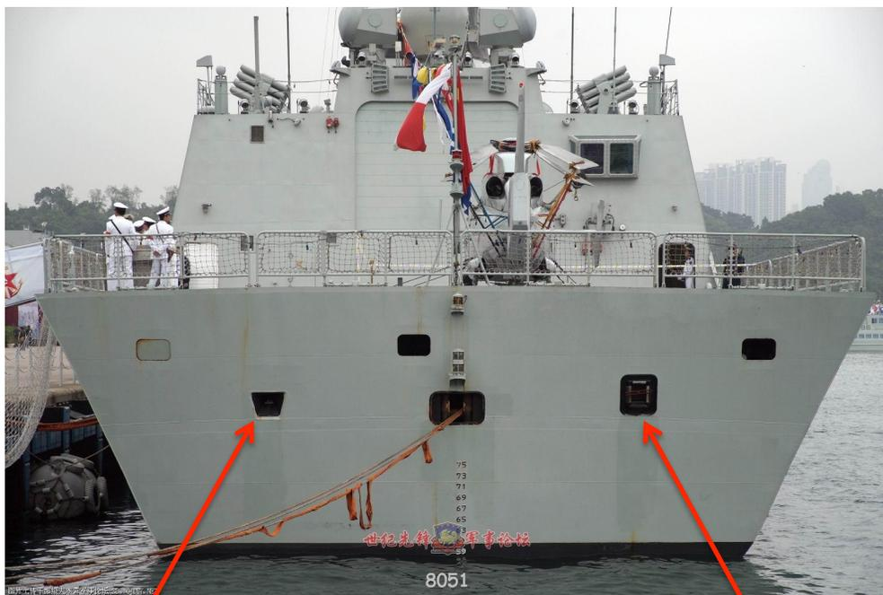
The Type 054A frigate has two deployment ports for the towed array and the acoustic torpedo decoy. Chinese websites have identified the starboard opening as the one for deploying the towed array. The port opening is described as the one used by the towed torpedo decoy.
