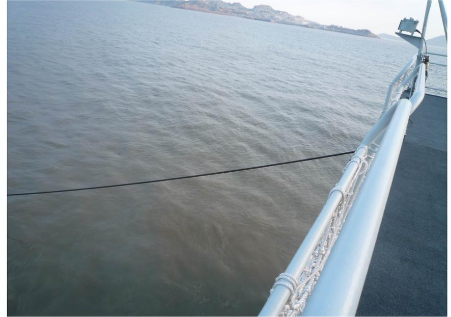
Photography of a Type 054A frigate with a streamed tow cable has recently been seen on Chinese websites. The accompanying discussions on the blog sites state this is evidence of a towed array.
